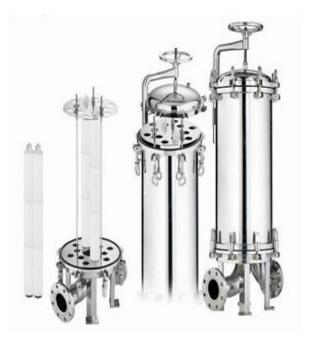
Head: 316L Stainless Steel Bowl: 316L Stainless Steel Center Post with Seal plate: 316L SS Vent/ Drain Plug: 316L Stainless Steel O-Rings: Silicone, Viton or EPDM
